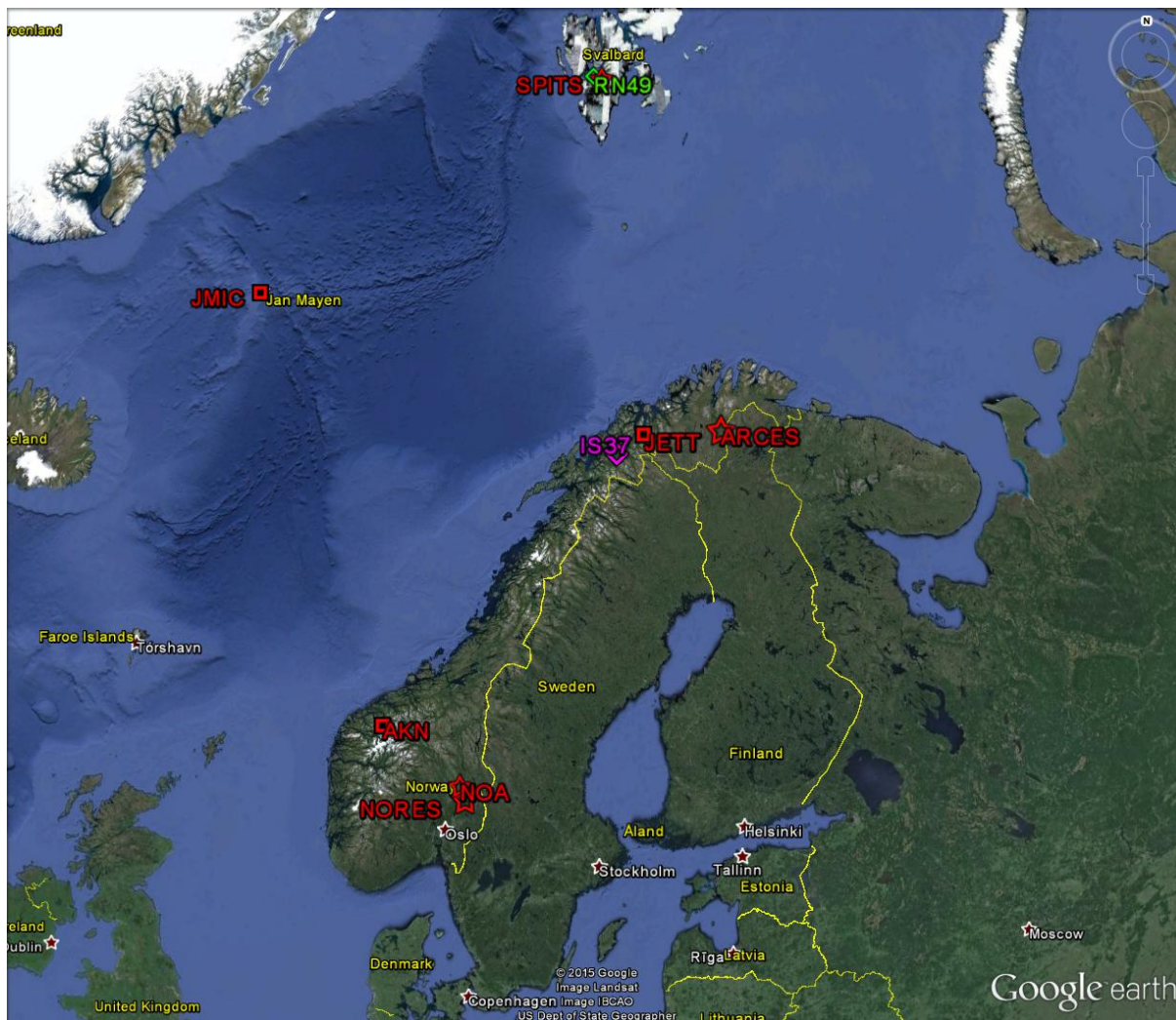
Figure 2. A map of the Norwegian IMS stations, the NORES array and the two 3C stations AKN and JETT. NORSAR, as the Norwegian NDC, is responsible for the seismic auxiliary stations AS72 (SPITS array) and AS73 (3C stations JMIC), the primary stations PS27 (NOA array) and PS28 (ARCES array), the infrasonic array (I37NO), and the radionuclide station on Spitsbergen (RN49). NOA is the array with the largest aperture of the whole IMS network.
