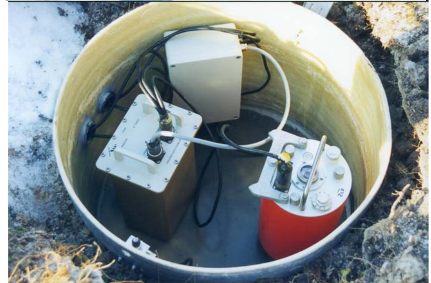
ARCES array. There are no boreholes. Only small vault to house the equipment.
